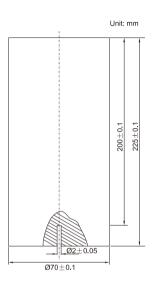
The test block is used to determine sensitivity margins of straight probe and instrument's comprehensive performances, to adjust sensitivity of flaw detection, to determine sizes of defects and to determine performances indicators and their shapes, e. g. vertical linearity, of instrument
